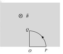
loop is then rotated counterclockwise with a uniform angular velocity  $\omega$  about an axis perpendicular to the paper passing through the point O.
